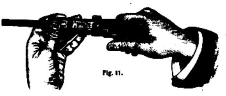
(see fig. 11) can fall into its place in front of the hooks of the recoil spring bell crank with which the breech mechanism engages, when pressed back.
